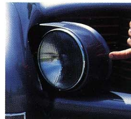
Curved vanes (above) to reduce wheelhouse turbulence normally hide behind the front fender skirts of B.A.T. 5 (below). Headlamps (right) fold into the fenders.
