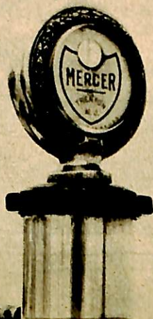
Mercer radiator cap contains a "Motometer" which registers the heat of the engine coolant.
