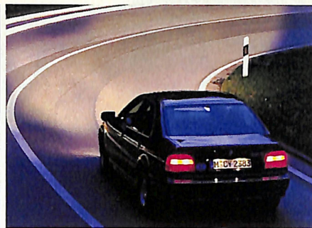
■ Bosch's seven-source headlamp assembly can broadly vary its beam pattern just by switching on or off individual lights. BMW's solution (above) actually swivels the headlamps' reflectors.
