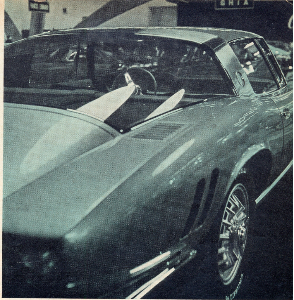
Iso A-3/L "Grifo" carries Bertone coachwork, as does standard 2+2. Headlights swing forward when in use.
