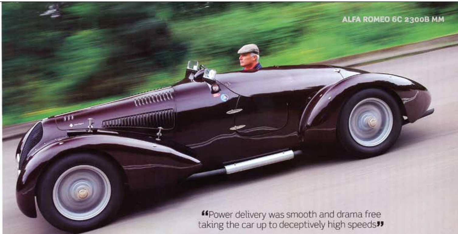
ABOVE: With just the driver in the car, a body-coloured alloy cover can be fitted over the passenger area
