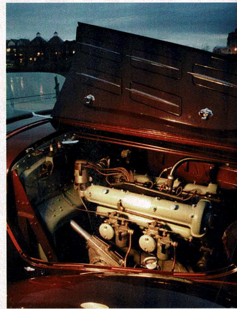
Clockwise, from below: straight-sided cockpit feels like a speedboat; twin Solex carbs raised twin-cam's power to 95bhp; engine's forward position dictated styling of 6C-2300; Mussolini's chauffeur Boratto en route to 13th place on the 1936 Mille Miglia
