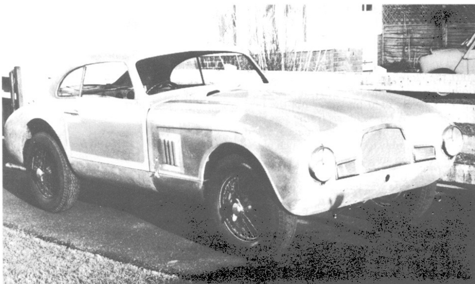
In the restoration, new bonnet panels were fabricated by Aubrey Fineburgh of Classic Autos.
