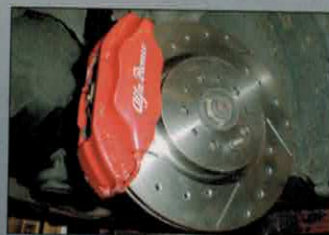
Drilled and Grooved
