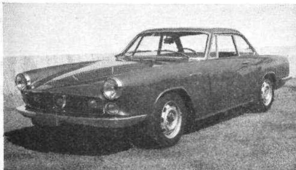
IT'S A FIAT. —Abarth have now turned their attention to the amelioration of the Fiat 2100. Fitted with three Weber carburettors, Dunlop disc brakes and a handsome four-seater body, the Fiat-Abarth 2200 is capable of speeds in excess of 120 m.p.h. and will be seen in England for the first time at the Earls Court Show.
