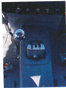
Above: beauty dictated more by function than by form. Left: Colombo's potent 3.0-liter V-12, topped by six dual-throat Weber 38 DCNs. Below: The GTO was Ferrari's first GT to use a shift gate.
