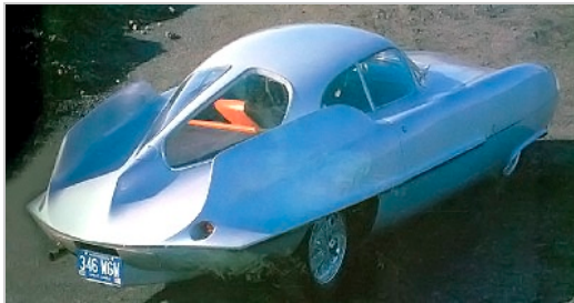
The 1955 Alfa Romeo Bertone BAT 9's body sides were free of air scoops and extractors. ©2007 Publications International, Ltd.
