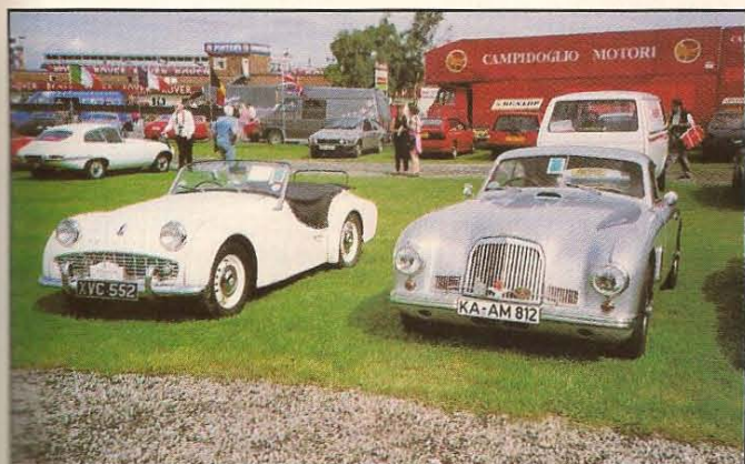
Above, the DB2 had a 'top-hat' grille instead of DB1's three-piece arrangement. This DB2 belongs to Tom Barnard's sister Left, when LML/50/8 was found it had a Mercedes-Benz engine
