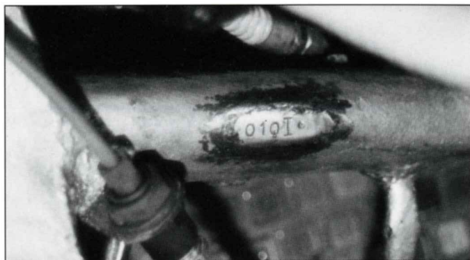
This is the frame of the Troubetzkoy car showing the serial "0101". This number was stamped in a soft non ferrous metal which had been poured onto the frame tube in a slight depression. Note that the "1" does not match the other numbers in size or angle.
