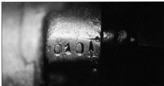
Serial number stamped in the rear of the engine block of 0101. The numbers have obviously been over stamped and there is evidence of filing. While the existing number is 0101, it is not clear what the underlying original number might have been.
