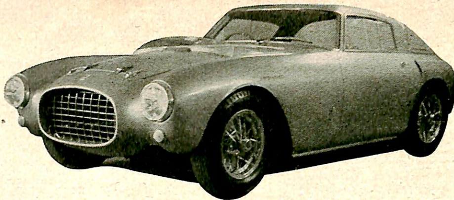
THREE-LITRE FERRARI: The latest Farina-bodied Type 250 "Mille Miglia" Ferrari has a V12 engine giving a guaranteed bench-test figure of 240 b.h.p.
