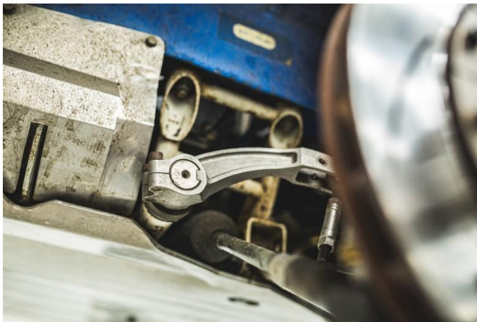
Original front cross member and roll bar
