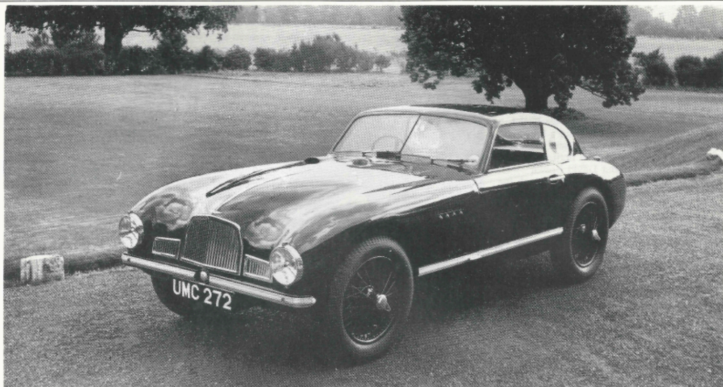
A very early pre-production car which was raced by Lance Macklin privately. The lines are more akin to the 1949 Le Mans race cars than the 1950 production car. Note louvres in wings and early three piece grille.
