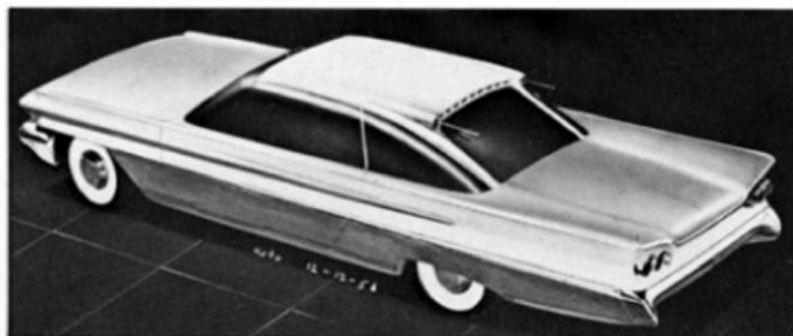
Models in 1/10th scale were photographed and airbrushed like this one, which shows rear treatment similar to 1959 Buick and Chevrolet.
