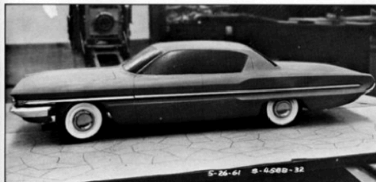
The 1/10th clays were (and still are) modeled against a mirror so only half needs to be done. Note camera reflected in background.
