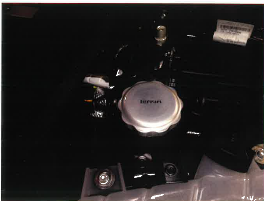
Serbatoio olio Oil tank
