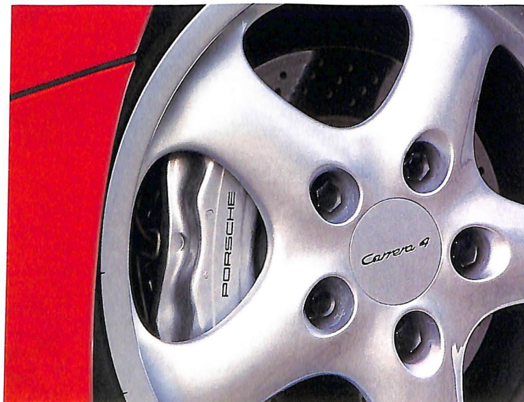
► Overeager driver inputs to the C4's honking cross-drilled brakes get ameliorated by 3-channel Bosch ABS 5.
